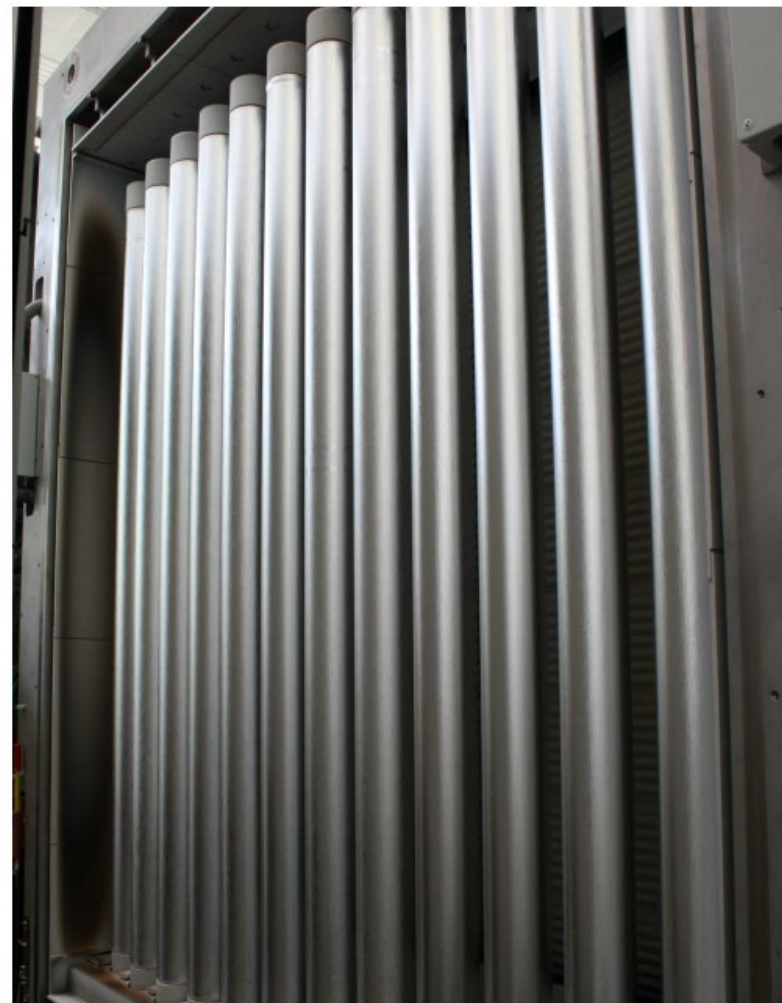
Figure 1: Rotary target array consisting of 12 Gen8.5 Al5N targets installed at PiVot™ sputter system.
